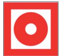
F08 Brandmelder (manuell)
